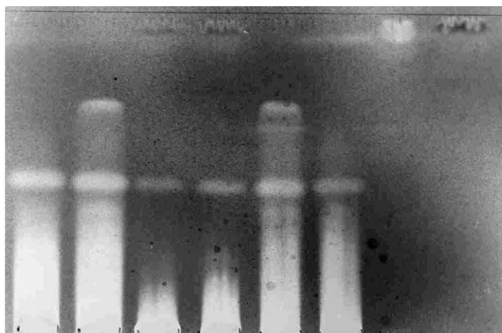
Fig. 3: Chromatogram of 100 µg of bark (B), root (R) and leaf (L) extracted by ethanol (Eth), acetone (Ac), hexane (Hx) and dichloromethane (Dc) separated by EMW and sprayed with DPPH reagent. Light areas indicate anti-oxidant activity. Lanes from left to right R-Eth, B-Eth, L-Eth, L-Ac, B-Ac, R-Ac, L-Hx and L-Dc.
