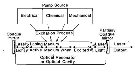
Fig. 1:Mechanism of laser light production (modified from Bailin et al.4)
